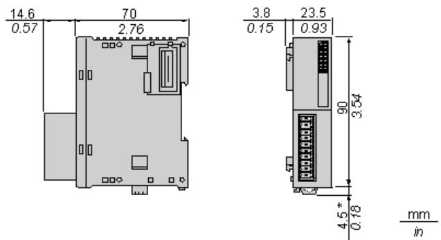
NOTE: \* 8.5 mm (0.33 in) when the clip-on lock is pulled out.
