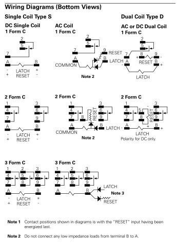
Note 3 Resistor and diodes connected by customer. See Coil Data Chart on KUL Series engineering data page for resistor value. Recommended using 1N4007 diode.
