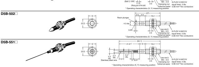
Note: 1. Unless otherwise specified, a tolerance of ±0.4 mm applies to all dimensions.
