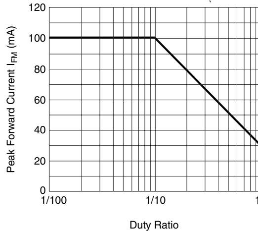
Fig. 2 Peak Pulsed Forward Current I FM vs. Duty Ratio
