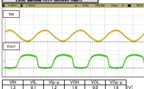
Typical sample at Vcc=5V,25deg.C      Vertical: 1V/div., Horizontal: 100ns/div.
