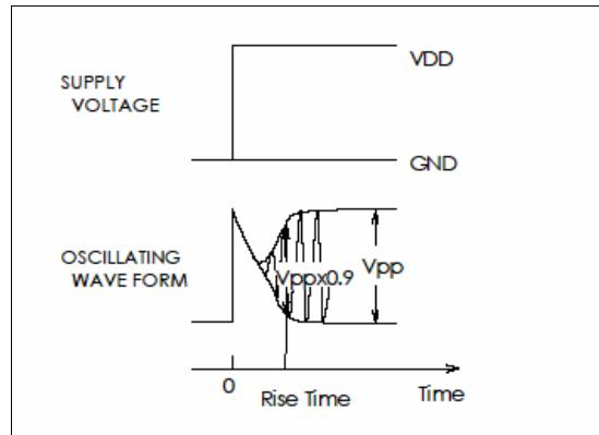
In the case that rising time of supplied voltage ( $V_{dd}$  or  $V_{set}$ ) is slower than that of resonator, resonator's rise time depends on that of power supply.
