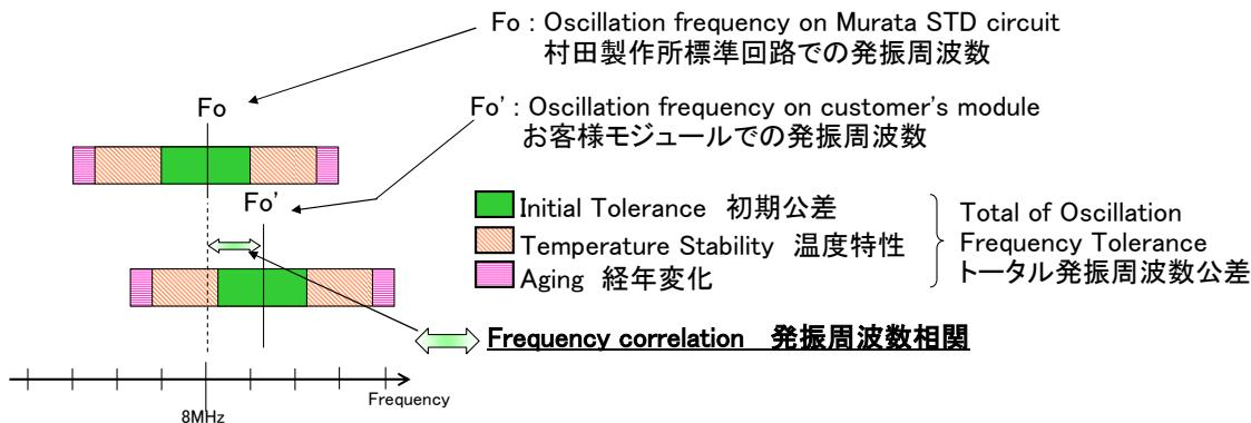
To meet required oscillation frequency tolerance, we would like to offer customized part number with frequency adjusted on your final PCB.
