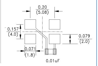
**Note**: It is recommended to use an approximately 0.01uF bypass capacitor between PIN 2 and 4.
