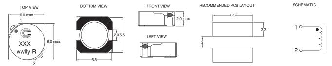
Dimensions are in millimeters.
