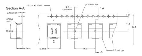
Supplied in tape-and-reel packaging, 950 parts per reel, 13" diameter reel.
