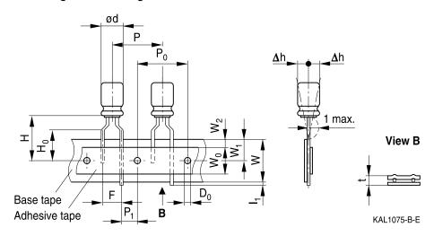
Lead spacing 5.0 mm (from d  $\times$  I = 10  $\times$  12.5 mm to 12.5  $\times$  30 mm) Last 3 digits of ordering code: 008
