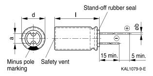
Safety vent for diameter  $\geq$  6.3 mm.
