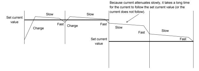
If RNF, current watching point, was the set current value (output current) in the mixed decay mode and in the fast decay mode, there is no charge mode but the slow + fast mode (slow to fast is at MDT) in the next chopping cycle.
