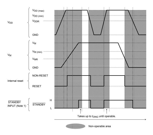
Note 1: If the V<sub>DD</sub> drops to the level of the V<sub>DDR</sub> or below while the specified voltage is input to the V<sub>M</sub> pin, the IC is internally reset.
