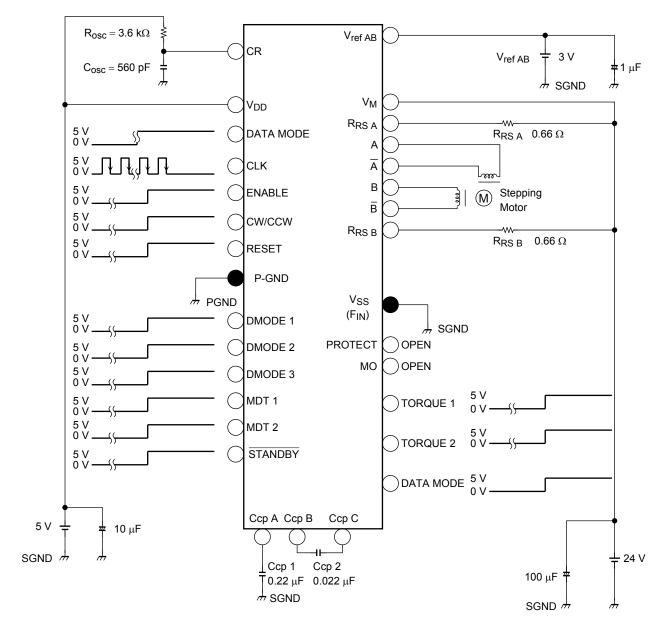
Note: Adding bypass capacitors is recommended.
