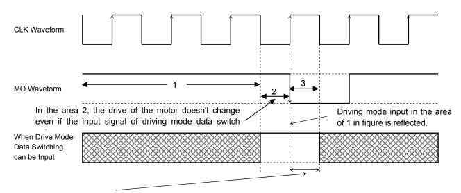
During MO output (phase data halted: the area of 3 above) to forcibly switch drive modes, a function to set RESET = High and to initialize the electrical angle is required.
