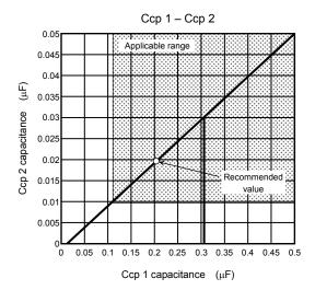
Choose Ccp 1 and Ccp 2 to be combined from the above applicable range. We recommend Ccp 1:Ccp 2 at 10:1 or more. (If our recommended values (Ccp1 =  $0.22~\mu F$ , Ccp 2 =  $0.022~\mu F$ ) are used, the drive conditions in the specification sheet are satisfied. (There is no capacitor temperature characteristic as a condition.)
