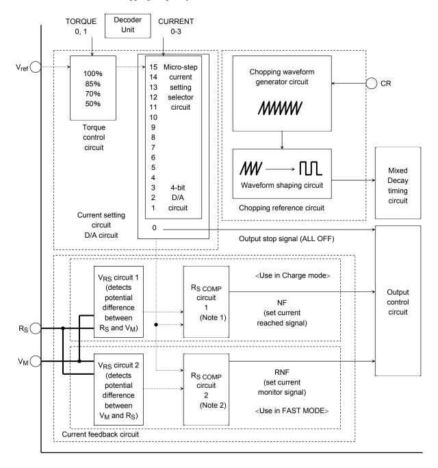
Note 1: R<sub>S COMP1</sub>: Compares the set current with the output current and outputs a signal when the output current reaches the set current.
