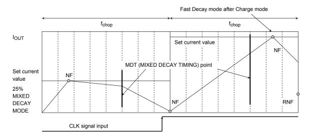
• In MIXED DECAY MODE, when the output current > the set current value
