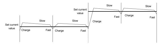
• Sine wave in decreasing (When using MIXED DECAY Mode with large attenuation ratio (MDT%) at attenuation)
