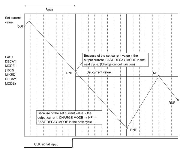
The output current to the motor is in supply voltage mode after the current value set by  $V_{\rm ref}$ ,  $R_{\rm RS}$ , or Torque reached at the set current value.
