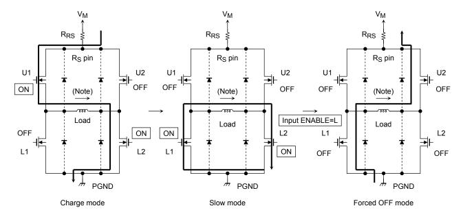
As shown in the figure at above, an output transistor has parasitic diodes.
