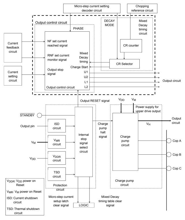
Note: The STANDBY pins are pulled down in the IC by 100-k $\Omega$  resistor. When not using the pin, connect it to GND. Otherwise, malfunction may occur.
