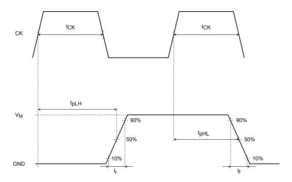
Figure 1 Timing Waveforms and Names
