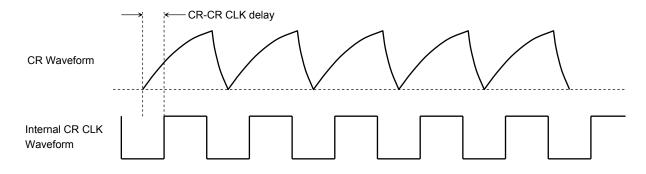
Figure 2 Timing Waveforms and Names (CR and output)
