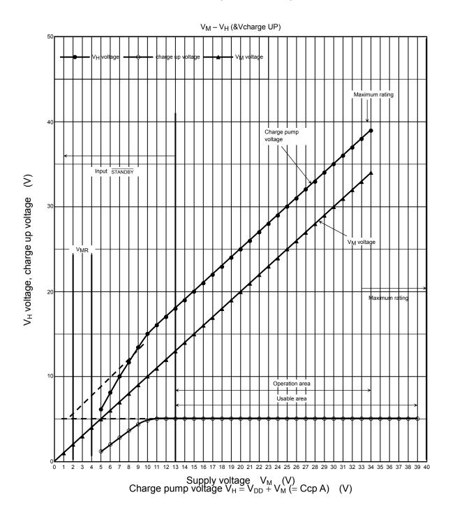
Note:  $V_{DD}=5~V$   $Ccp~1=0.22~\mu F,~Ccp~2=0.022~\mu F,~f_{Chop}=150~kHz$ (Be aware the temperature changes of capacitance of charge pump capacitor.)
