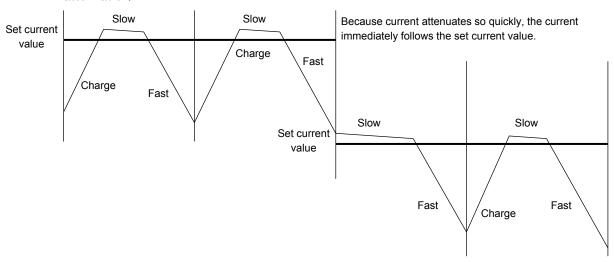
$\circ$  Sine wave in decreasing (When using MIXED DECAY Mode with small attenuation ratio (MDT%) at attenuation)
