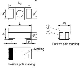
① Encapsulation: molded epoxy resin
