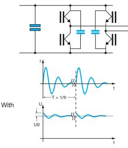
L = stray inductance IGBT + capacitor R = serial resistance IGBT + capacitor
