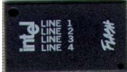
Figure 2. Mark for Pin-1 indicator on 48-Lead 8Mb, 16Mb and 32Mb TSOP
