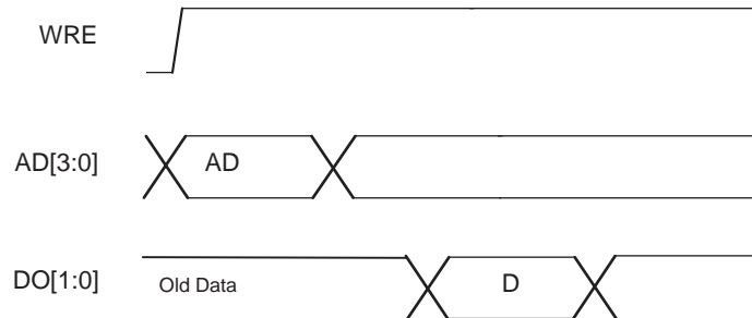
Figure 3-7. Slice Single /Dual Port Read Cycle Timing
