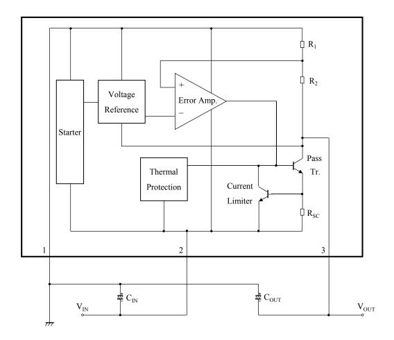
$C_{\rm IN}~$ : When a wiring from a smoothing circuit to a three-pin regulator is long, it is likely to oscillate at output. A capacitor of 0.1  $\mu F$  to 0.47  $\mu F$  should be connected near an input pin.
