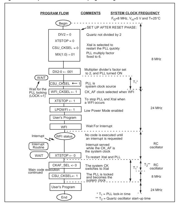
Figure 38. Example of Low Power Mode programming
