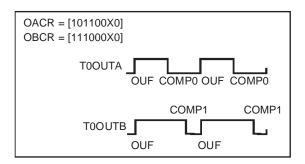
For a configuration where TxOUTA is driven by the Over/Underflow, by Compare 0 and by Compare 1; TxOUTB is driven by both Compare 0 and Compare 1. OACR is programmed with TxOUTA preset to "0". OUF toggles Output 0, as do CM0 and CM1. OBCR is programmed with TxOUTB preset to "1". OUF does not affect the output; CM0 resets TxOUTB and CM1 sets it.
