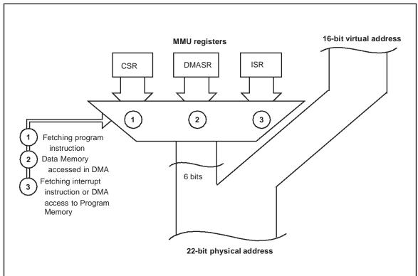
Figure 17. Addressing via CSR, ISR, and DMASR
