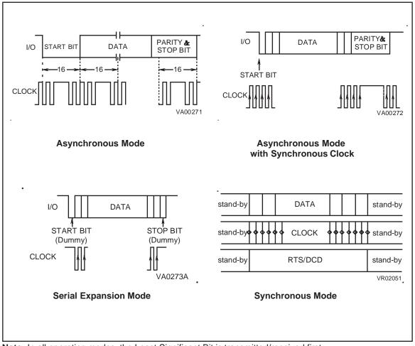
Note: In all operating modes, the Least Significant Bit is transmitted/received first.
