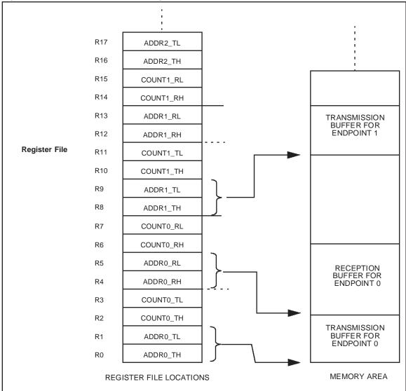
Figure 70. DMA buffers and related register file locations
