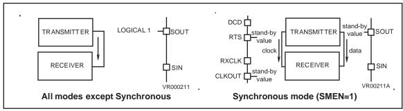
Figure 78. Auto Echo and Loop-Back Configuration
