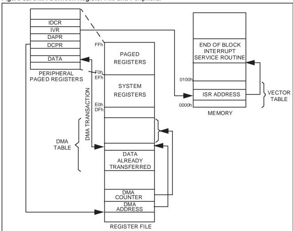
Figure 32. DMA Between Register File and Peripheral
