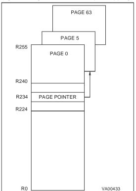
Figure 10. Addressing the Register File
