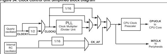
Figure 34. Clock Control Unit Simplified Block Diagram
