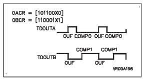
For a configuration where TxOUTA is driven by the Over/Underflow and by Compare 0, and TxOUTB is driven by Compare 0 and 1. OACR is programmed with TxOUTA preset to "0". OUF sets TxOUTA, CM0 resets it and CM1 has no effect. OBCR is programmed with TxOUTB preset to "0". OUF has no effect, CM0 sets TxOUTB and CM1 toggles it.
