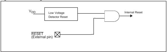
Figure 48. Low Voltage Detector Reset Signal
