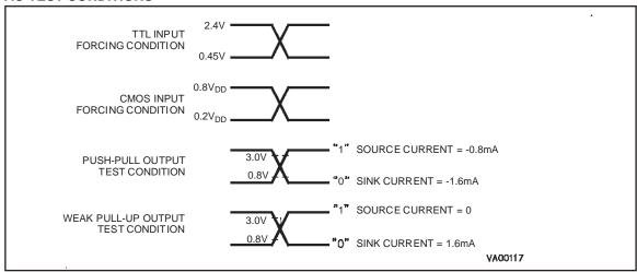
$<sup>^{(2)}</sup>$  External pull-up (1.5 Kohms connected to USBV<sub>CC</sub>); Operating conditions: V<sub>DD</sub> = 4.0 - 5.25V ; T<sub>A</sub> = 25°C
