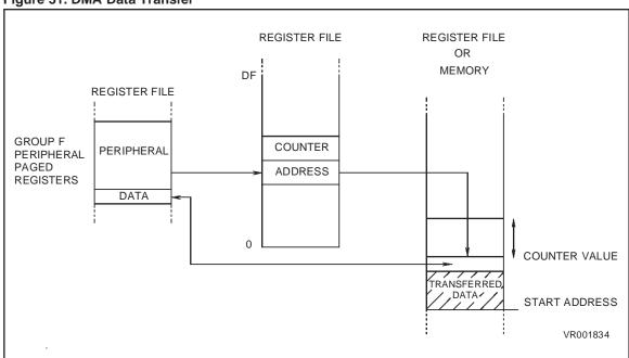
Figure 31. DMA Data Transfer
