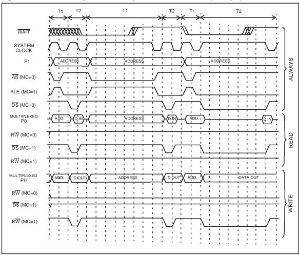
Figure 52. External memory Read/Write sequence with external wait (WAIT pin)
