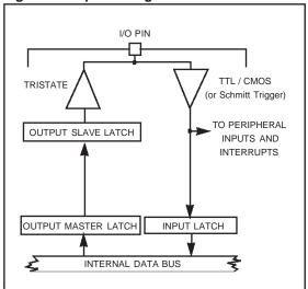
Figure 58. Output Configuration
