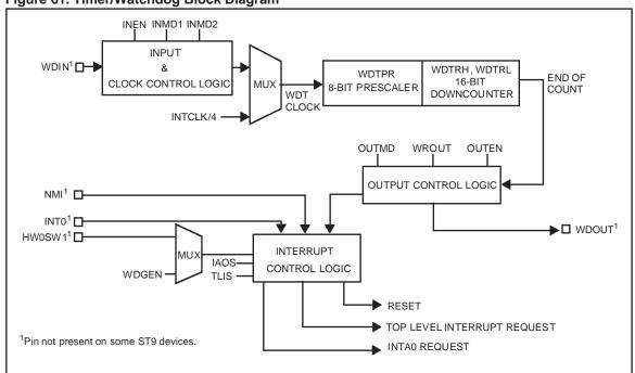
Figure 61. Timer/Watchdog Block Diagram
