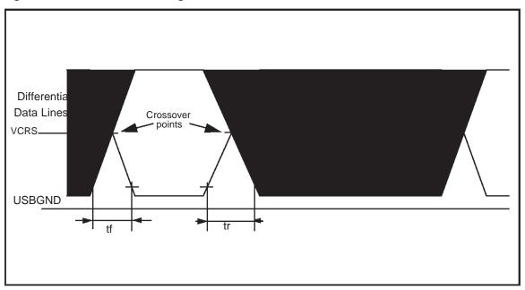
**USB INTERFACE: FULL SPEED CHARACTERISTICS** ( $V_{DD} = 4.0 - 5.5V$ ,  $T_A = 0^{\circ}C + 70^{\circ}C$ , unless otherwise specified)
