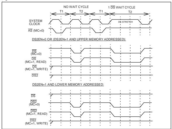
Figure 51. External memory Read/Write with a programmable wait
