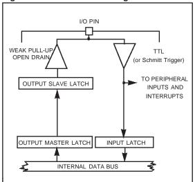
Figure 60. Alternate Function Configuration
