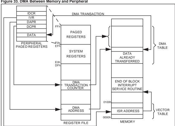
Figure 33. DMA Between Memory and Peripheral
