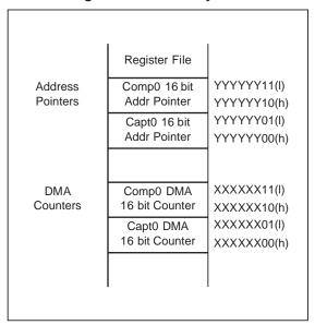
Figure 68. Pointer Mapping for Register to Register Transfers
