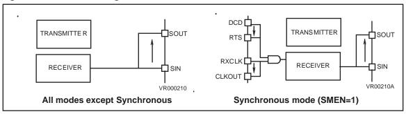
Figure 77. Loop Back Configuration
