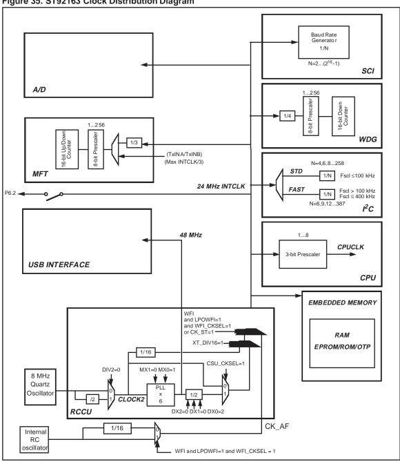
Figure 35. ST92163 Clock Distribution Diagram
