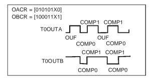
For a configuration where TxOUTA is driven by the Over/Underflow and by Compare 0, and TxOUTB is driven by the Over/Underflow and by Compare 1. OACR is programmed with TxOUTA preset to "0". OUF sets TxOUTA while CM0 resets it, and CM1 has no effect. OBCR is programmed with TxOUTB preset to "1". OUF toggles TxOUTB, CM1 sets it and CM0 has no effect.
