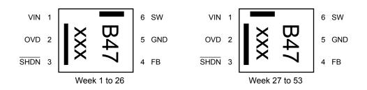
Note: This IC could be destroyed in some case if amounted in 180° inverse direction. Please be careful about IC direction in mounting.
