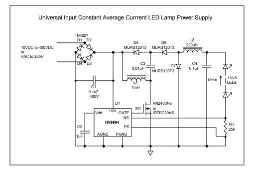
This circuit provides a constant average current output, which may be used to power LED lamps. The circuit maintains a constant average current and the value of C4 capacitor controls the peak-topeak ripple, which decreases with increasing capacitor value. If
