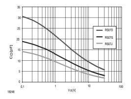
Figure 3. Typ. Diode Capacitance vs. Reverse Voltage
