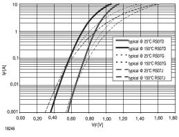
Figure 1. Typical Forward Characteristics
