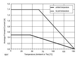
Figure 2. Forward Current Derating Curve
