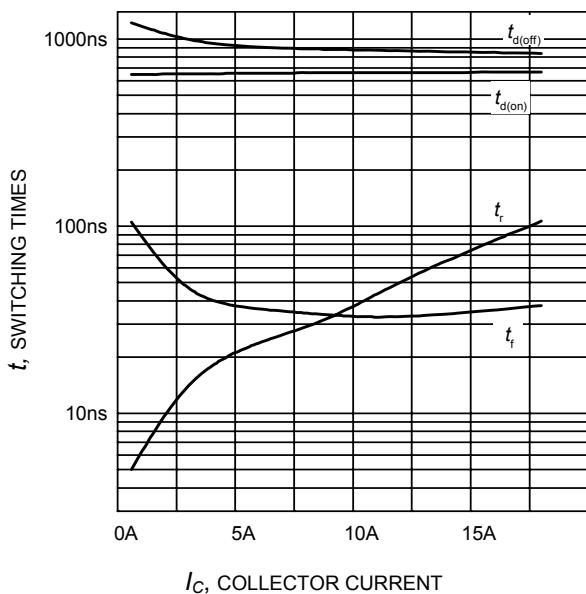
**Figure 5.** Typical switching times as a function of collector current
