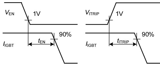
**Figure C: Definition of Enable and ITIRP propagation delay**
