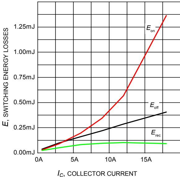
**Figure 7.** Typical switching energy losses as a function of collector current
