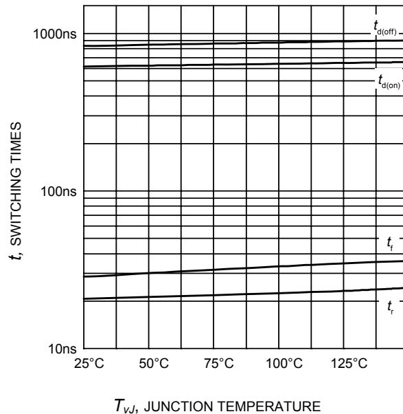
**Figure 6.** Typical switching times as a function of junction temperature
