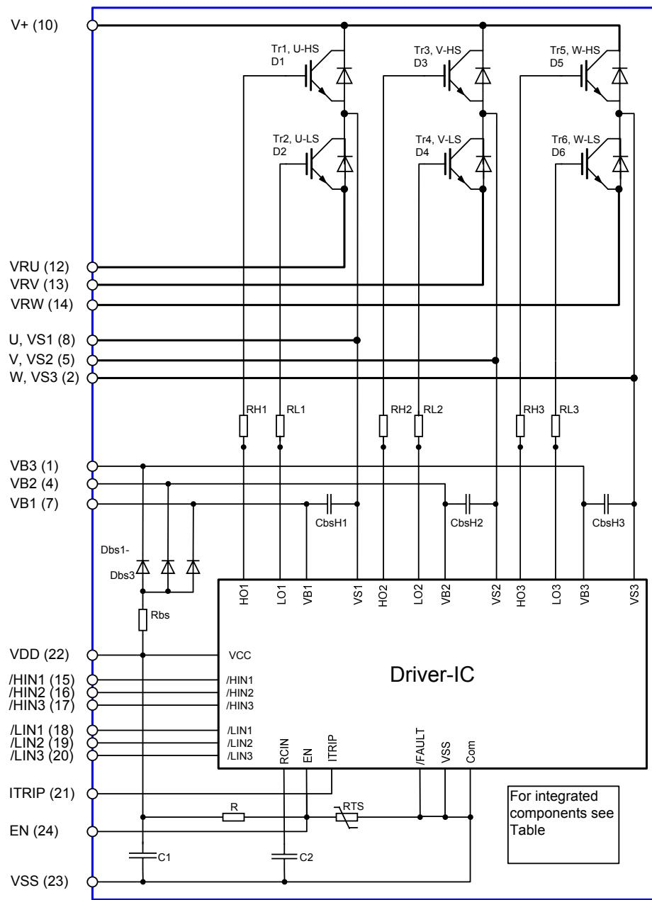
**Figure 1: Internal Schematic**
