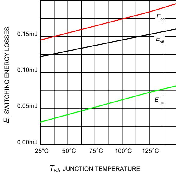
**Figure 8.** Typical switching energy losses as a function of junction temperature
