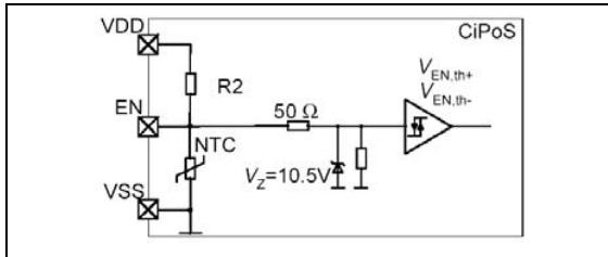
**Figure 3: Internal Circuit at pin EN**
