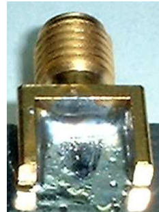
Figure 19. Soldering details of connector fingers to lower ground plane.
