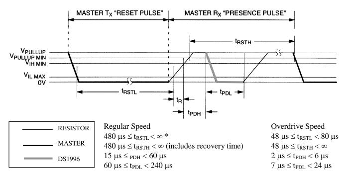
\* In order not to mask interrupt signaling by other devices on the 1-Wire bus,  $t_{RSTL} + t_R$  should always be less than 960 µs.
