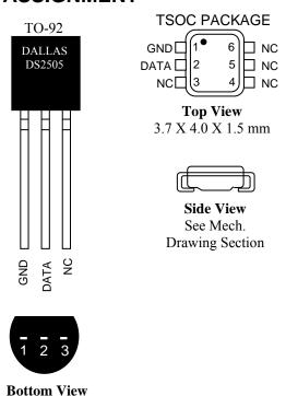
**NOTE:** The leads of TO-92 packages on tapeand-reel are formed to approximately 100 mil (2.54 mm) spacing. For details see the *Package Information* section.
