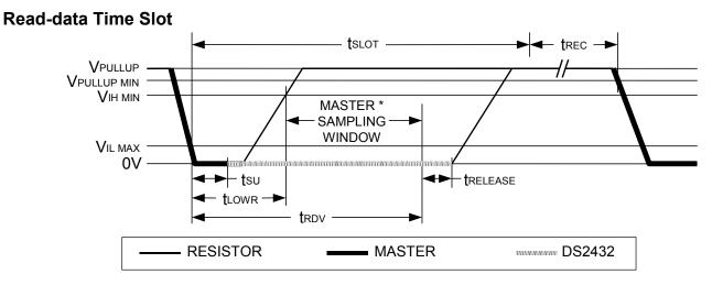
\*The optimal sampling point for the master is as close as possible to the end time of the  $t_{RDV}$  period without exceeding  $t_{RDV}$ . For the case of a Read-one time slot, this maximizes the amount of time for the pullup resistor to recover the line to a high level. For a Read-zero time slot it ensures that a read will occur before the fastest 1-Wire device releases the line ( $t_{RELEASE} = 0$ ).
