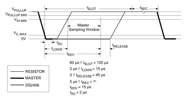
\* The optimal sampling point for the master is as close as possible to the end time of the  $15\mu s$   $t_{RDV}$  period without exceeding  $t_{RDV}$ . For the case of a Read-one time slot, this maximizes the amount of time for the pull-up resistor to recover the line to a high level. For a Read-zero time slot it ensures that a read will occur before the fastest 1-Wire devices(s) release the line ( $t_{RELEASE} = 0$ ).
