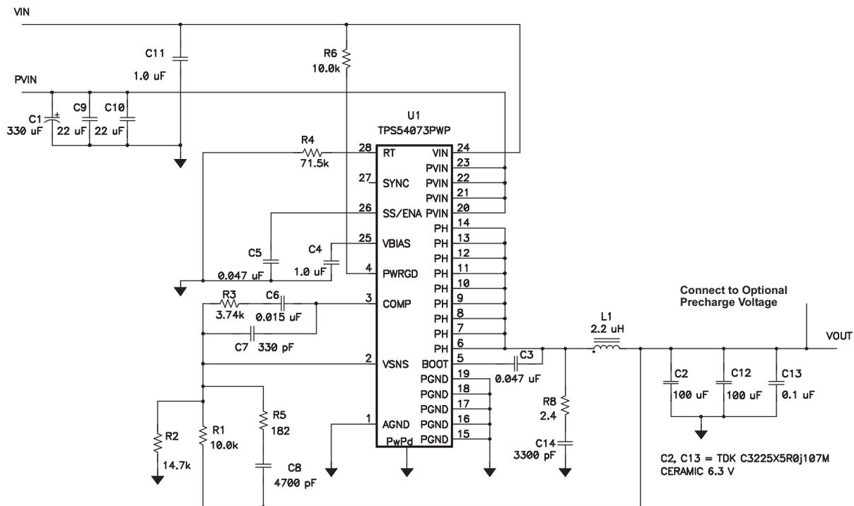
Figure 13. 1.5 V Power Supply With Ceramic Output Capacitors
