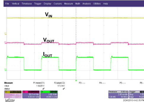
Load Transient (Sink test)
