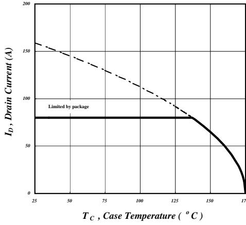
**Fig 11. Maximum Continuous Drain Current v.s. Case Temperature**
