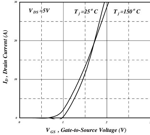
**Fig 11. Transfer Characteristics**
