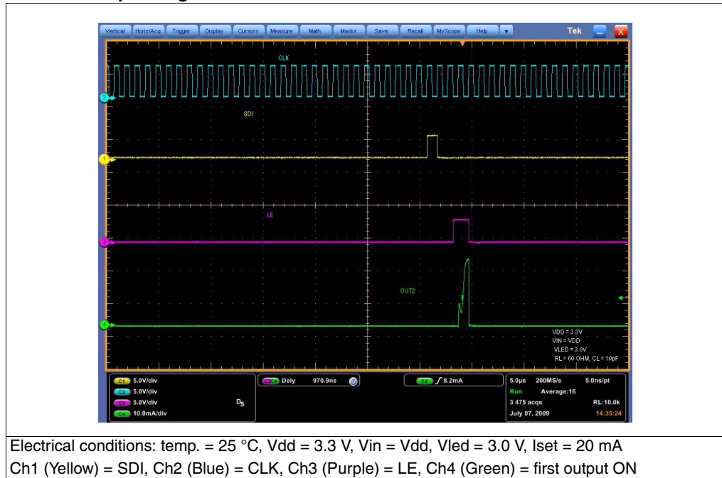
Figure 19. First output ON after switching from auto power saving to normal operating condition
