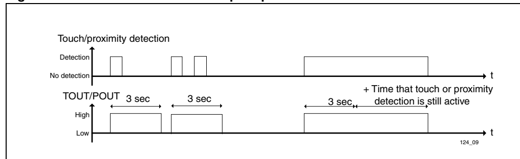
Figure 14. 3-second latch mode output operation
