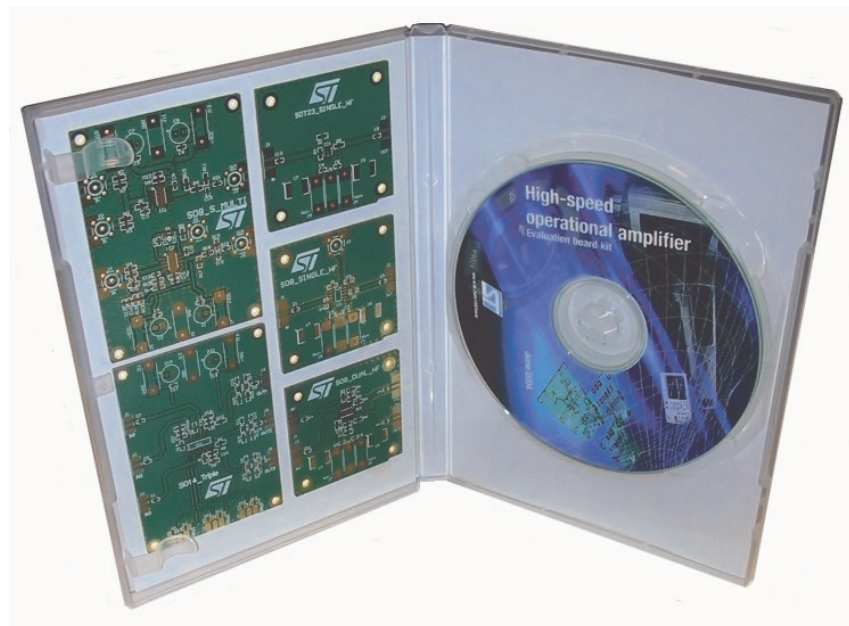
Figure 30. Evaluation kit for high-speed op-amps
