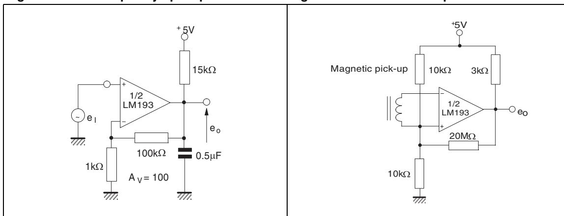
Figure 12. Transducer amplifier
