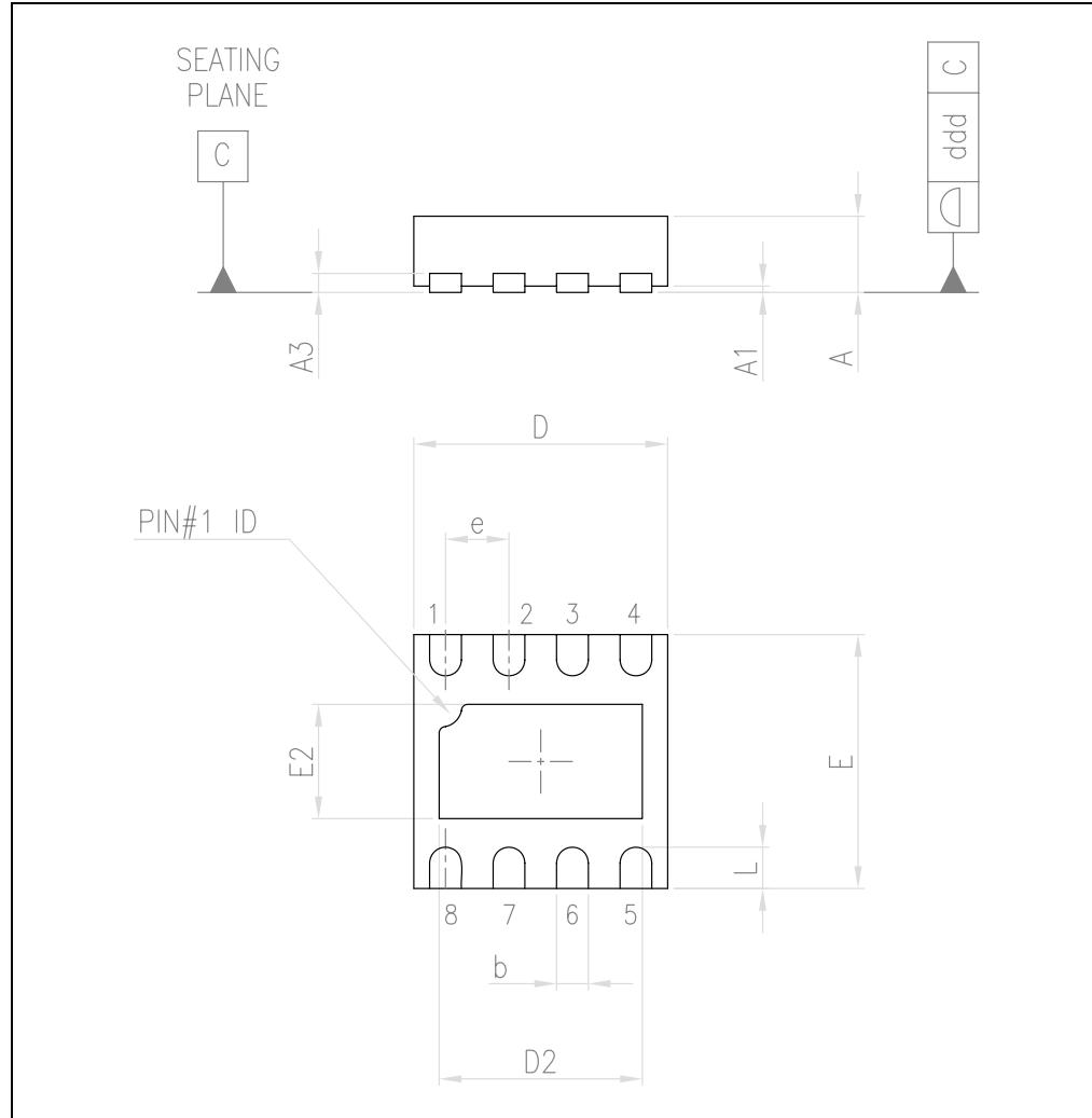
**Table 8. DFN8 2x2x0.6 mm package mechanical data (pitch 0.5 mm)**
