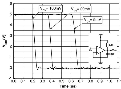
**Figure 6. Response time for various input overdrives - positive transition**
