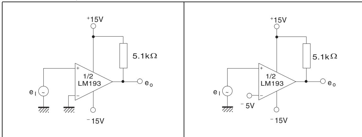
**Figure 18. Comparator with a negative reference**
