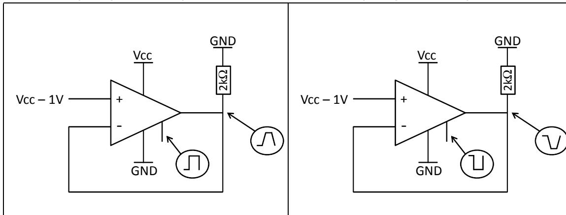
**Figure 23.** Turn-on time,  $V_{\text{CC}} = 5 \text{ V}$ , Vout pulled down,  $T = 25^\circ \text{ C}$
