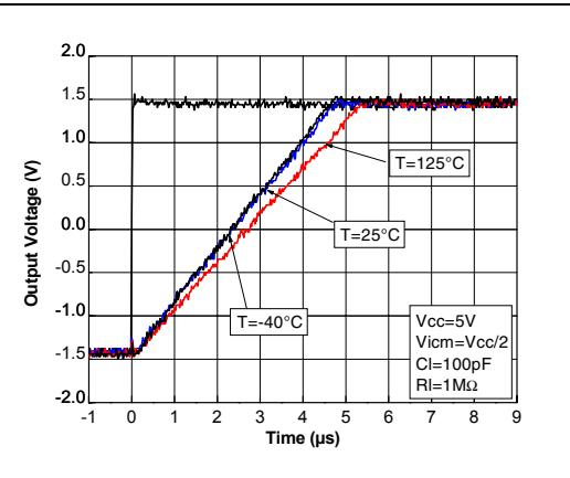
**Figure 16. Negative slew rate at  $V_{CC} = 5$  V with  $C_l = 100$  pF**
