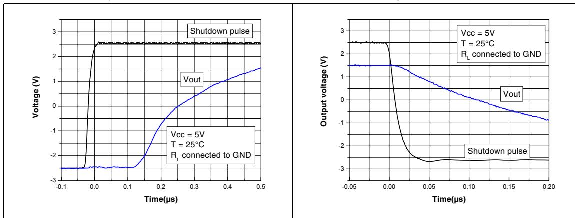
**Figure 24.** Turn-off time,  $V_{\text{CC}} = 5 \text{ V}$ , Vout pulled down,  $T = 25^\circ \text{ C}$
