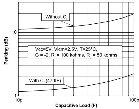
Another way to improve stability and reduce peaking is to add a capacitor in parallel with the feedback resistor. As shown in *Figure 16*, the feedback capacitor drastically reduces the peaking versus capacitive load (inverting gain configuration, gain = -2).
