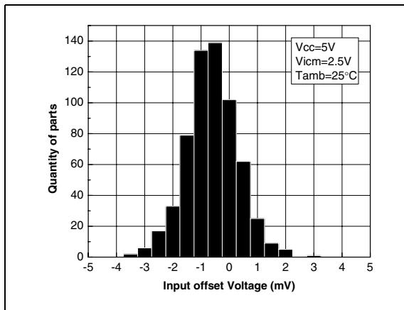
**Figure 2. Input offset voltage distribution at  $T = 125^\circ\text{C}$**
