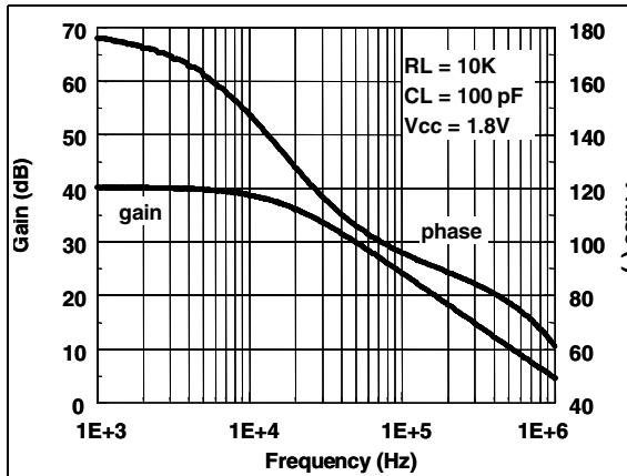
**Figure 26. Gain and phase vs. frequency at  $V_{cc} = 3$  V**
