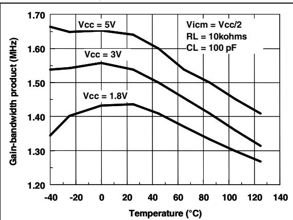
**Figure 29. Gain bandwidth product vs. supply voltage**
