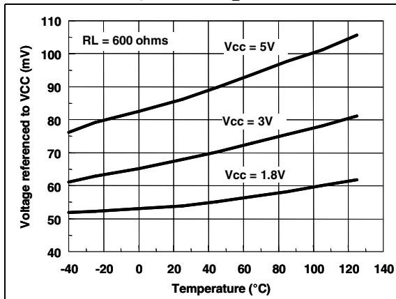
**Figure 16. Low level output voltage vs. temperature,  $R_L = 600\Omega$**
