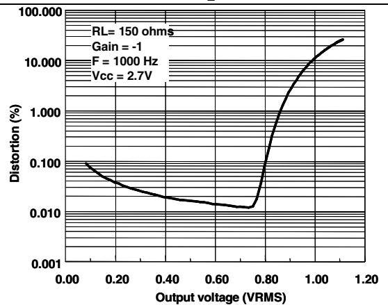
**Figure 41. Distortion vs. output voltage at V<sub>cc</sub> = 2.7 V, R<sub>L</sub> = 1500 Ω**
