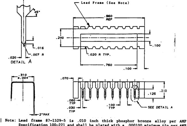
Note: Lead frame 8/-1529-5 is .010 inch thick phosphor bronze alloy per AMP Specification 100-221 and shall be plated with a .000100 minimum tin per AMP Specification 112-16-3. After plating, dummy IC module shall be cut from strip and formed as indicated.
