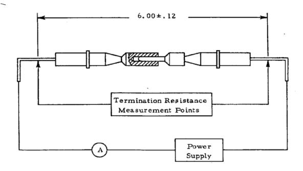
Note: Termination resistance equals millivolts divided by test current less resistance of 6 inches wire.
