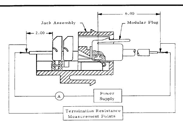
Note: Millivolt drop (resistance) due to the 6 inch and 2 inch wire lengths shall be subtracted from all readings.
