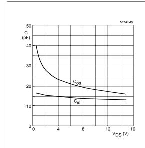
$V_{GS}$  = 0; f = 1 MHz;  $T_j$  = 25 °C.
