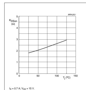
Drain-source on-state resistance as a function of junction temperature; typical values.
