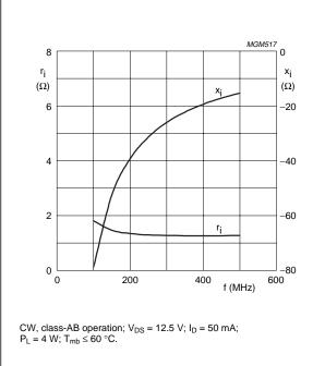
Fig.12 Input impedance as a function of frequency (series components); typical values.
