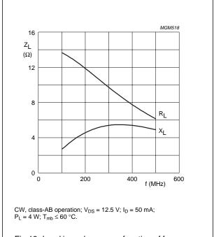
Fig.13 Load impedance as a function of frequency (series components); typical values.
