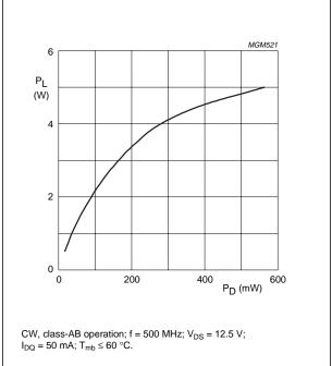
Fig.9 Load power as a function of drive power; typical values.
