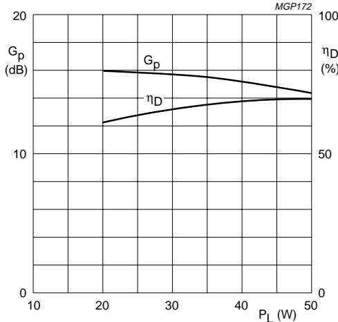
Class-B operation;  $V_{DS} = 28$  V;  $I_{DQ} = 50$  mA;
