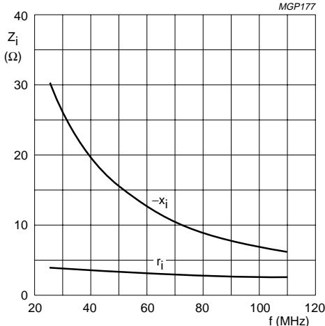
Class-B operation;  $V_{DS} = 28$  V;  $I_{DQ} = 50$  mA;
