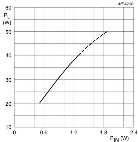
Class-B operation;  $V_{DS} = 28$  V;  $I_{DQ} = 50$  mA;
