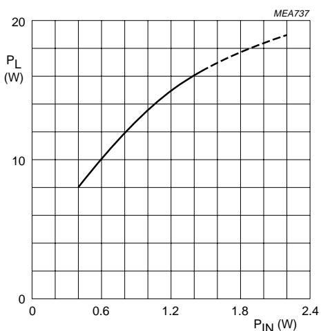
Class-B operation;  $V_{DS} = 12.5$  V;  $I_{DQ} = 50$  mA;
