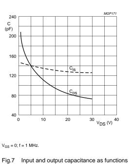
of drain-source voltage; typical values.
