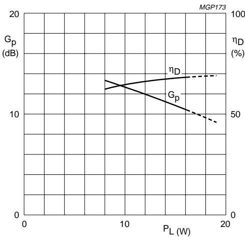
Class-B operation;  $V_{DS} = 12.5$  V;  $I_{DQ} = 50$  mA;
