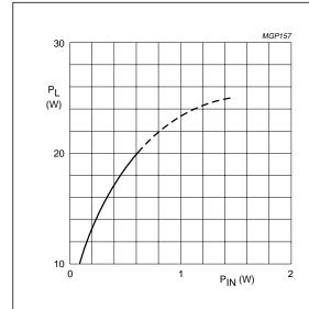
Class-B operation;  $V_{DS}$  = 28 V;  $I_{DQ}$  = 25 mA; f = 175 MHz;  $T_h$  = 25 °C;  $R_{th\ mb-h}$  = 0.3 K/W.
