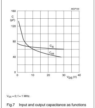
of drain-source voltage, typical values.
