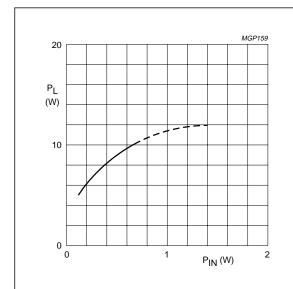
Class-B operation;  $V_{DS}$  = 12.5 V;  $I_{DQ}$  = 25 mA; f = 175 MHz;  $T_h$  = 25 °C;  $R_{th\ mb\text{-}h}$  = 0.3 K/W.
