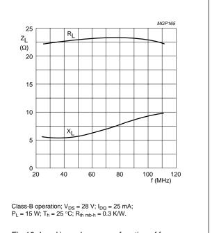
Fig.16 Load impedance as a function of frequency (series components); typical values.
