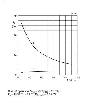
Fig.15 Input impedance as a function of frequency (series components); typical values.
