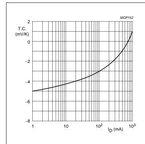
Fig.4 Temperature coefficient of gate-source voltage as a function of drain current, typical values.
