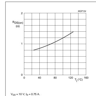
Drain-source on-state resistance as a function of junction temperature, typical values.
