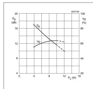
Class-B operation;  $V_{DS}$  = 12.5 V;  $I_{DQ}$  = 25 mA; f = 175 MHz;  $T_h$  = 25 °C;  $R_{th\ mb-h}$  = 0.3 K/W.
