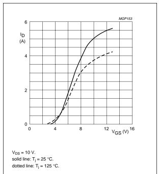
Fig.5 Drain current as a function of gate-source voltage, typical values.
