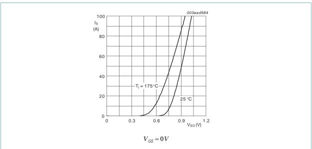
Fig 17. Source (diode forward) current as a function of source-drain (diode forward) voltage; typical values
