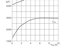
Fig 6. Input and reverse transfer capacitances as a function of gate-source voltage; typical values
