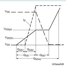
Fig 15. Gate charge waveform definitions
