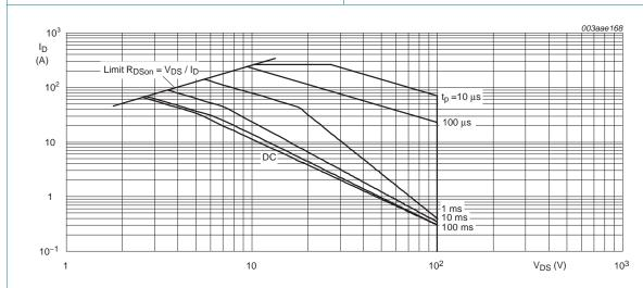
$T_{mb}$  = 25 °C;  $I_{DM}$  is a single pulse
