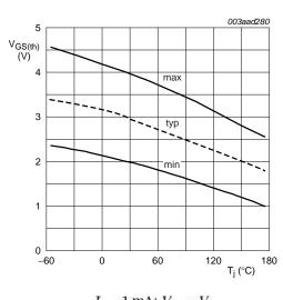
$I_D = 1 \text{ mA}; \ V_{DS} = V_{GS}$
