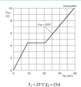
Fig 14. Gate-source voltage as a function of gate
