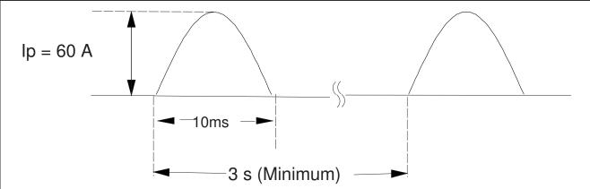
Fig.1. Repetitive surge conditions.  $I_P=60A$  (f=50Hz) at  $Tc=45^{\circ}C$ . Maximum number of cycles n=100k. Repetitive cycle T=3 seconds minimum.
