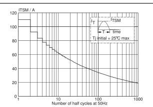
Fig.5. Maximum permissible non-repetitive peak on-state current  $I_{TSM}$ , versus number of cycles, for sinusoidal currents, f = 50 Hz.
