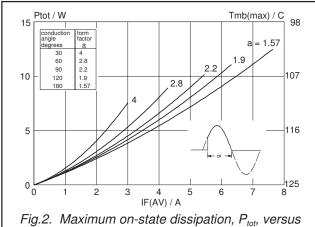
Fig.2. Maximum on-state dissipation,  $P_{tot}$ , versus average on-state current,  $I_{T(AV)}$ , where  $a = form \ factor = I_{T(RMS)} / I_{T(AV)}$ .
