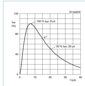
Fig 1. 8/20 µs pulse waveform according to IEC 61000-4-5
