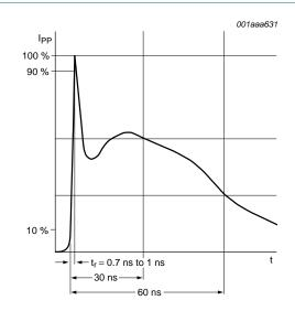
Fig 2. ESD pulse waveform according to IEC 61000-4-2
