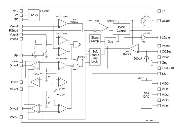
Figure 1 - Simplified block diagram of the US3027.
