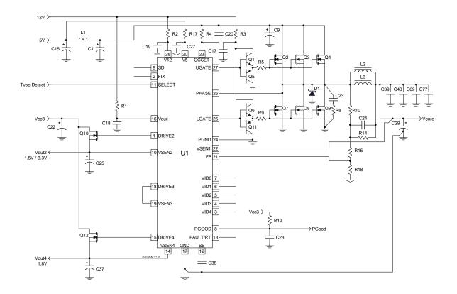
Figure 2 - Typical application of US3027 for the AMD Slot A socket
