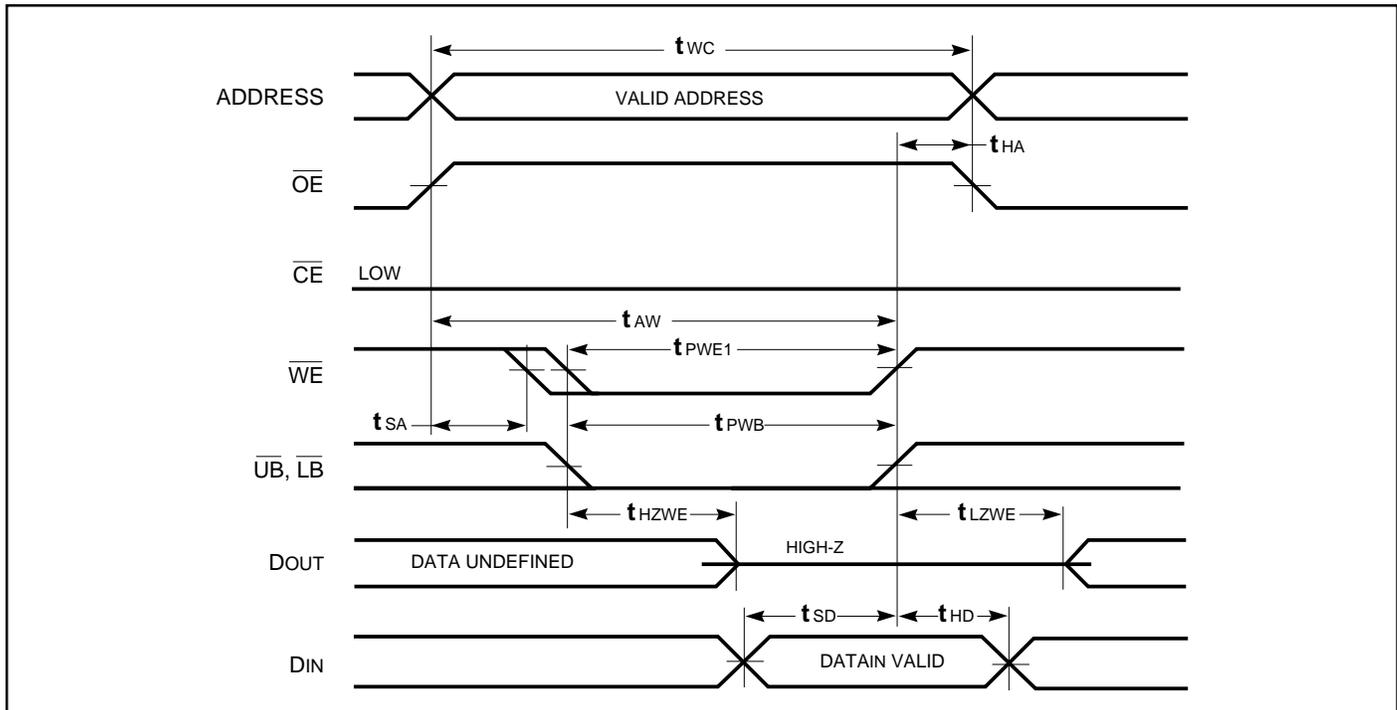
WRITE CYCLE NO. 3 ( $\overline{WE}$  Controlled.  $\overline{OE}$  is LOW During Write Cycle) <sup>(1)</sup>
