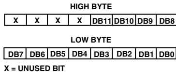
Figure 30. Data Format for AD5343
