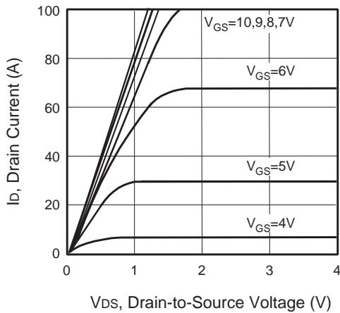
Figure 1. Output Characteristics
