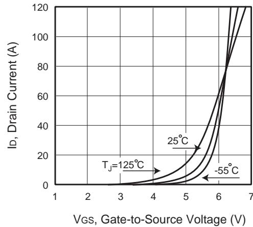
Figure 2. Transfer Characteristics
