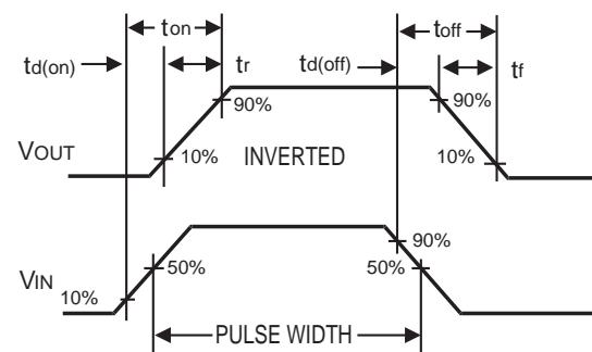
Figure 10. Switching Waveforms
