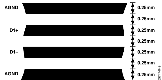
Figure 61. Arrangement of Signal Tracks
